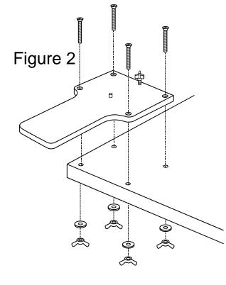
Mount to Table (hardware not provided) This is an alternate way to mount the base. Most customers use the portable version shown above
